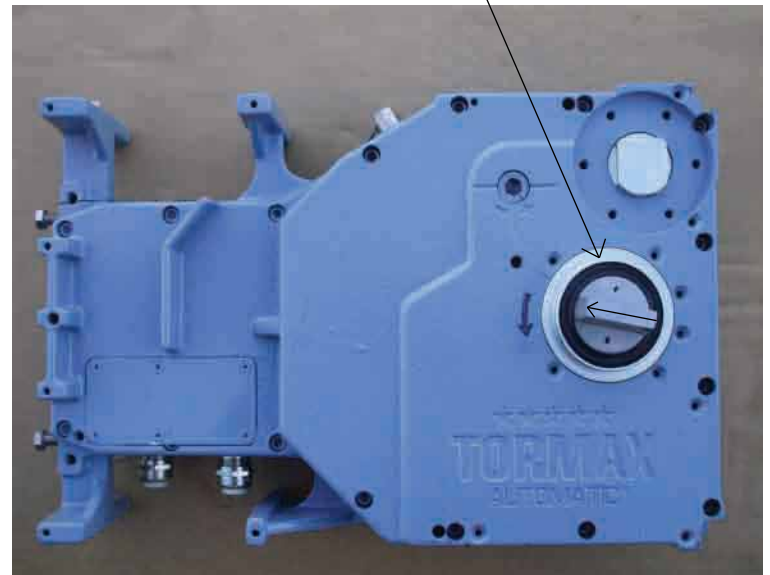
Position of shaft after 10 degree preload
